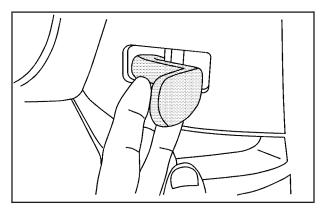
To tilt the wheel, hold the steering wheel and pull the lever toward you. Then move the wheel to a comfortable position and release the lever to lock the wheel in place.
