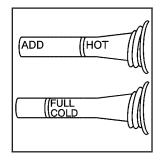
When the engine compartment is hot, the level should be at the HOT mark. When the engine compartment is cool, the level should be at the FULL COLD mark.
