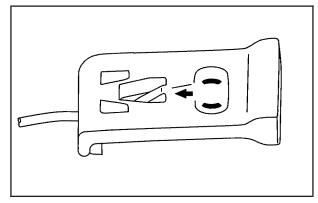
From outside the vehicle, use the door release tab located on the carpet inside the trunk on the driver's side of the vehicle. Pull the tab to unlock and unlatch the driver's door. See *Hatch/Trunk on page 2-14* for information on opening the trunk during a loss of power.
