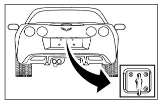
If your vehicle has lost battery power, open the hatch/trunk using the vehicle key. The key lock cylinder is located on the rear of the hatch/trunk lid above the license plate. Turn the vehicle key clockwise in the lock. If your vehicle has a convertible top and has lost battery power, you can also use the emergency trunk release handle to open the trunk. See "Emergency Trunk Release Handle" following.
