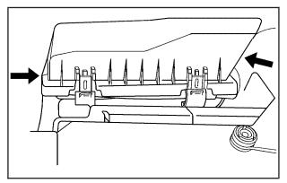
If you are cleaning your vehicle with the hood open, take care not to spray water directly into either end of the air cleaner/filter housing, as shown in the illustration, as this could damage your vehicle's engine.
