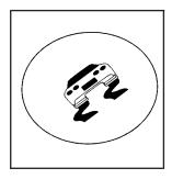
To turn the system off, press the button located on the console. You can turn the system on or off at any time by pressing the ACTIVE HANDLING button. The DIC will display the appropriate message when you push the button.
