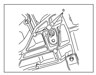
3. Lift the vehicle with the jack, making sure the jack spans at least two of the crossmember ribs (B).
