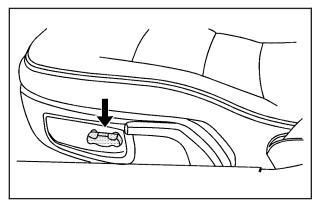
The control for the driver's power seat is located on the outboard side of the seat cushion. Your vehicle may also have a passenger power seat.
