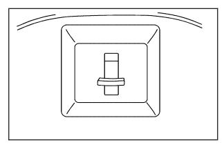
Both seatbacks fold forward to give you access to the rear area. To fold a seatback forward, lift this latch, which is located on top of the backside of the seat, and pull the seatback forward. The seatback will lock down in this position. To unlock, lift up on the latch and push the seatback rearward. When you return the seatback to its original position, make sure the seatback is locked in place.
