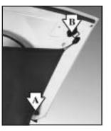
Hook the elastic loops on the front corners (A) of the shade to the T-nuts located on the front corners of the rear hatch frame.
