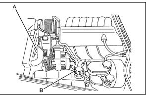
A. Electric Engine Cooling Fan
