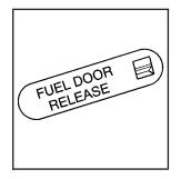
There is also a manual fuel door release tab. It is located against the upper trim in the rear compartment on the driver's side of the vehicle. Pull the tab to release the fuel door. Be careful not to spill fuel. Do not top off or overfill the tank and wait a few seconds after you have finished pumping before removing the nozzle. Clean fuel from painted surfaces as soon as possible. See *Washing Your Vehicle on page 5-86*.
