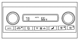
When your vehicle is first started, the display will show the driver's temperature setting, the outside temperature, the fan speed and the air delivery, for about 10 seconds.
