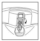
6. Push up on the handle of the rear roof release handle to latch its hook in the closed position.
