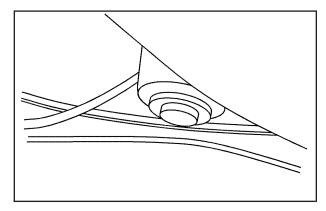
6. Tilt the driver's seatback forward and press the tonneau cover release button located on the underside of the tonneau cover (C) behind the driver's seat. Then raise the tonneau cover (C). If the tonneau cover does not release and three chimes are heard, check to make sure the trunk lid is closed. Also, the cover will not release if the vehicle alarm is turned on.
