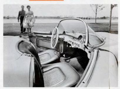
SECURITY AND LUXURY for driver and passenger are the keynotes of the snug Corvette cockpit. Individual bucket seats have form-fitting foam rubber cushions. The floor is covered in soft carpeting, backed by sponge rubber. Large pockets and ash trays in doors also serve as arm rests. Beautifully balanced instrument panel includes key-turn starter, electric clock, tachometer, hooded radio speaker.
