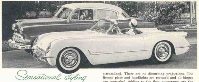
The low-set Corvette body expresses the swiftness that is so dramatically demonstrated by the car's performance. Taking full advantage of the new body material—glass-fiber reinforced plastic—Chevrolet engineers have created a sports car body in which all contours are smoothly
